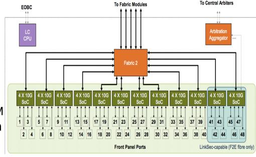
ASIC = application-specific integrated circuit, think 'small routing engine'
