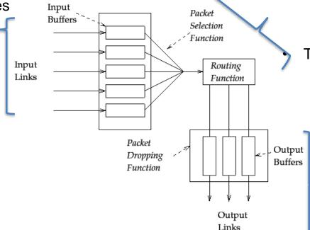
Figure 1: Basic Router Architecture
